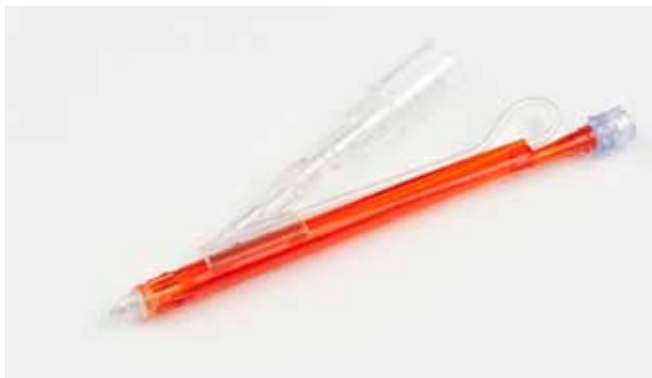
Fig. 3: The prototype handpiece with a backpack like opening for standard vials was used to test liquids having a higher viscosity. The system displayed does also have a triple outlet.
